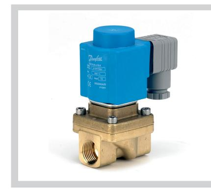
EV250B with assisted lift can operate from zero and up to 10 bar differential pressure. This 2/2-way valve program is especially to use in closed circuits with low differential pressure, but demanding moderate flow rates. Valve body in dezincification resistant brass for ensuring a long life even in connection with aggressive steam media.
